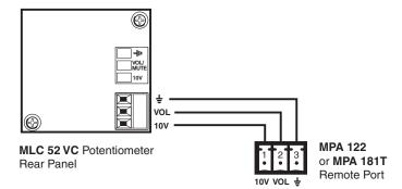
Wiring the VC potentiometer to the MPA remote volume control port
